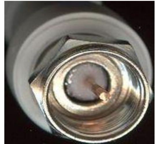
Male F-Connector, Connecting co-axial cable with the device
